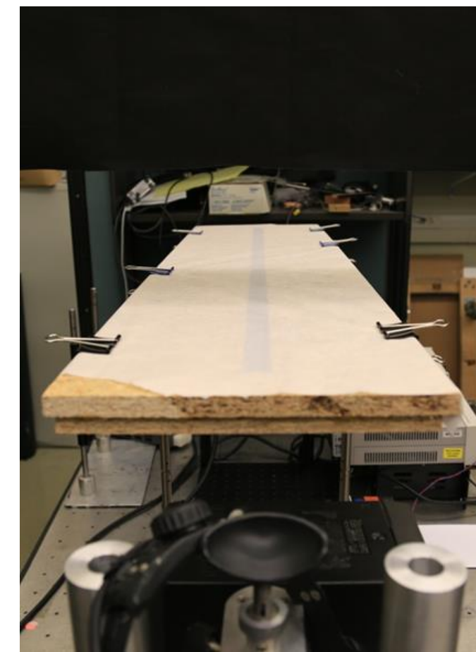
Figure 3. Vergence eye movement inducer. A laser dot was directed by a mirror galvanometer to appear on the board. The galvanometer would move the dot so it would come closer and further away from the viewer. As the viewer focused on the dot, their eyes would converge and diverge.
