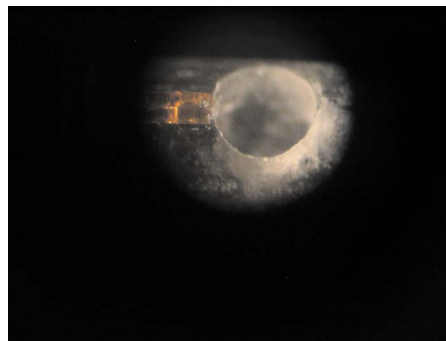
FIG. 1. (Color online) Photomicrograph of the port hole at distal tip of catheter, with a pair of 100\ \mu\text{m} diameter optical fibers positioned just at the left edge. The port hole is approximately 1 mm in diameter.
