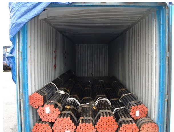
Figure 2.3. Unsecured steel pipe bundles
