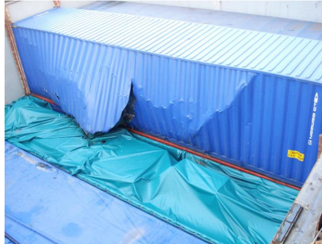
Figure 2.5. Side wall damaged
