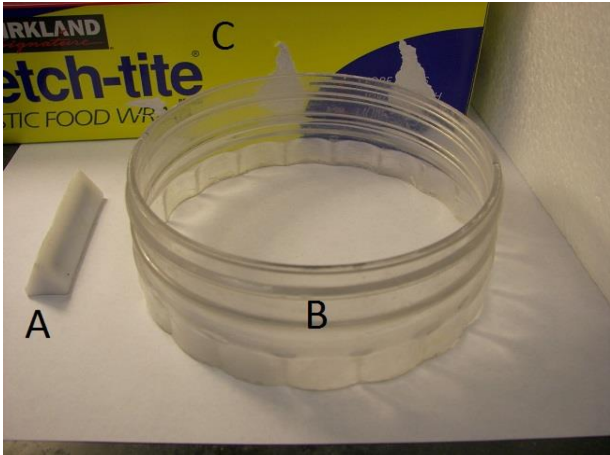
Figure 5 Plating Materials The materials needed for plating, including a triangular stirring rod (A), plastic ring (B), and polyethylene plastic wrap (C).
