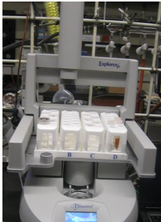
Figure 11. CEM Explorer 48 Microwave Reactor
