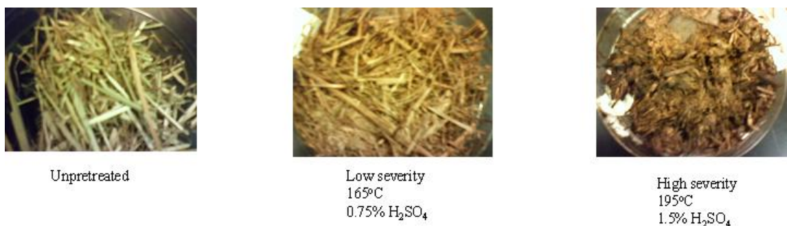
Figure 13. Switchgrass discoloration due to pretreatment
