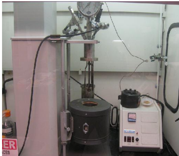
Figure 10. PARR ® High-Temperature, High-Pressure Reactor Model 4575A
