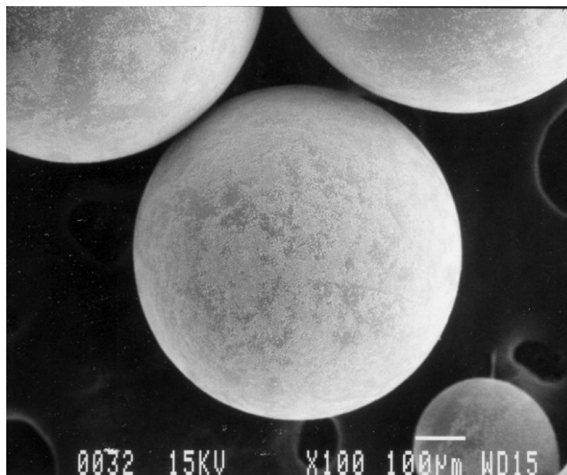
Fig. 3.5 Nanospheres on the surface of silica microspheres
