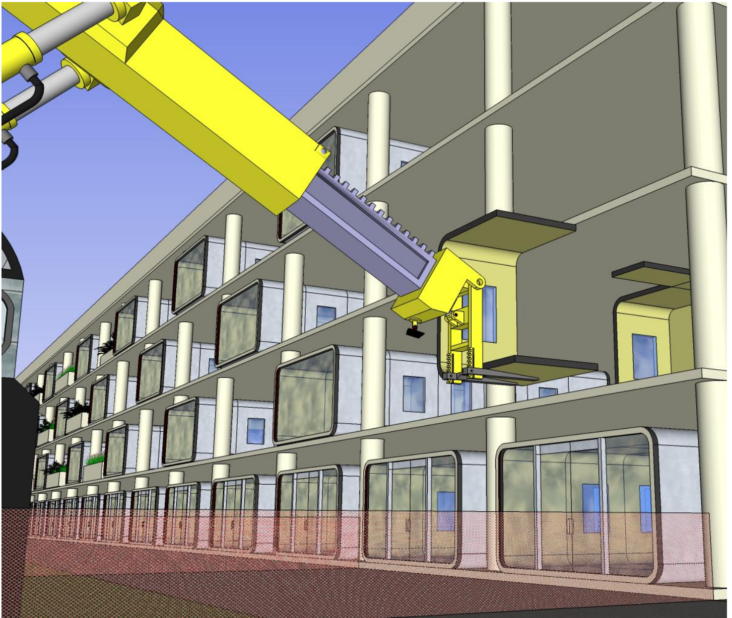
modular sections of the housing unit being placed in a parking structure
