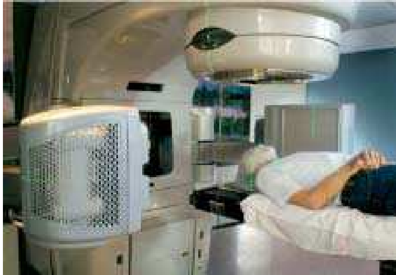
Figure 1.3 Example of Clinical setup with OBI. The system incorporates an x-ray tube and an amorphous-silicon flat-panel image detector on a pair of robotic arms.
