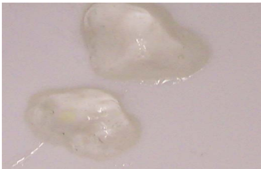
Figure 16. Appearance of G3-[PEG 12000-acrylate] 28 hydrogel after exposure to UV radiation
