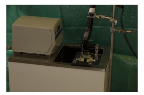
**Figure 2.1.** *Sonication Apparatus. A)* Custom-designed suspension platform for securing culture plates in the water bath and *B)* Sonication apparatus including suspension platform, water bath, laboratory stand and adjustable clamp holding the ultrasound transducer. This apparatus was used for all TUS exposures.
