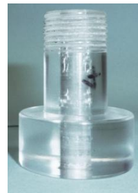
Figure 6.1 Inhalation flow cell design (A; schematic) and (B; photograph). Photographs in C show the top and the side views of the resistance tubes with identical external but different internal dimensions.
