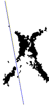
Figure 6.1: The wrong estimation of actual midpoint (straight line in the figure) based on minimal cut.
