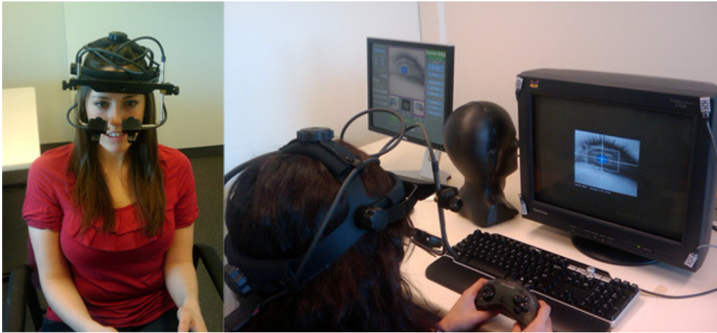
Figure 3. Pupil Cornea Eye tracking system. (from, “Eye Movement Monitoring of Memory”) 30
