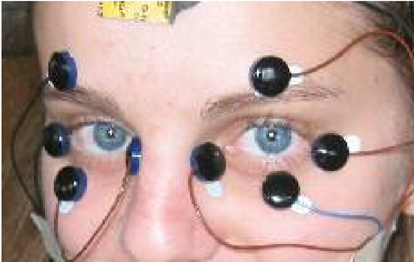
Figure 2. Placement of EOG surface electrodes around the eye. (from, “Metrovision: instruments for measuring eye movements”) 20
