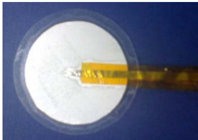
Figure 5-10 PVDF sensor incased in Mylar packaging
