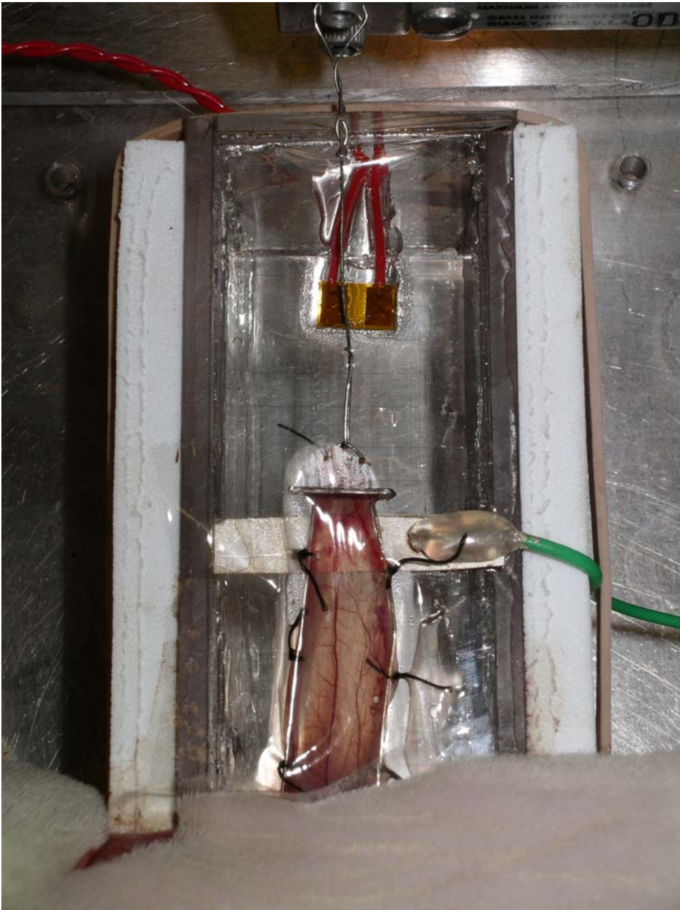
Figure 9. Spinotrapezius muscle on pedestal connected to force transducer and covered by Saran film.
