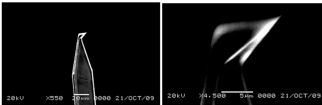
Figure 27 AC 160 cantilever before the nanoindentation experiments
