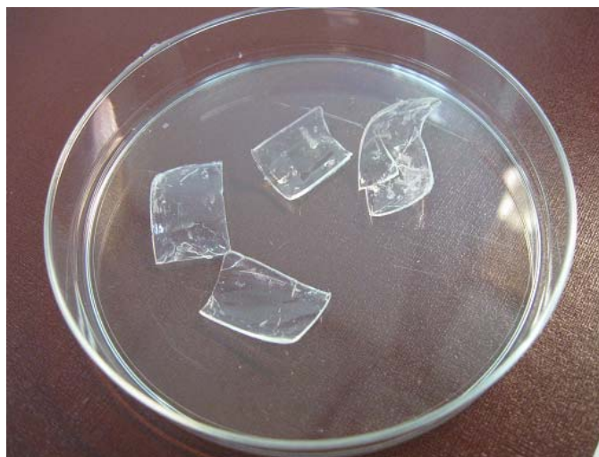
Figure 17 Examples of defective PEGDA samples
