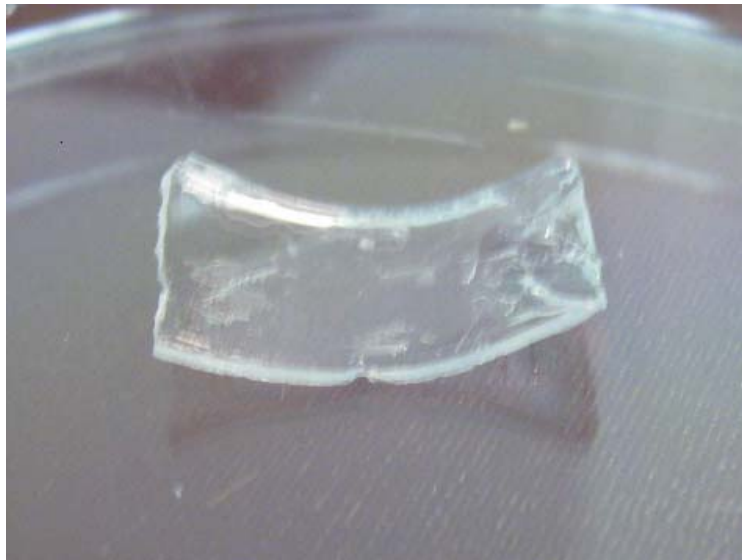
Figure 29 A deformed PEGDA hydrogel sample showing crack propagation
