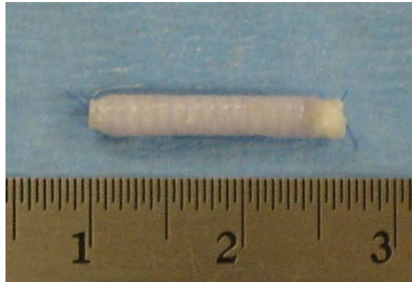
Figure 3.6. 1.8 mm I.D. reinforced PDO-elastin tube with imbedded PDS-II suture windings for possible use as a small-diameter vascular graft.
