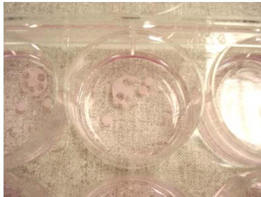
Figure 17. Photograph of the 3 mm biopsy punches taken from each scaffold disc for cell density, GAG, type I collagen and type II collagen, and histological analyses.
