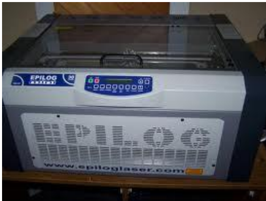
Fig. 2.6- CO 2 based laser system used to cut and ablate acrylic shims.
