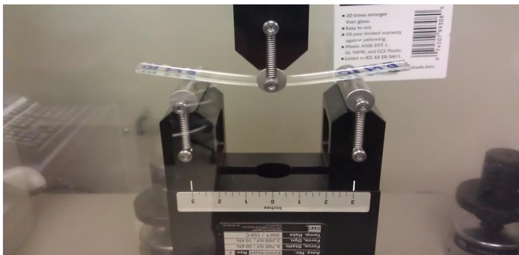
Fig. 2.11- One of the D790 3-point ASTM standard Bending test performed.
