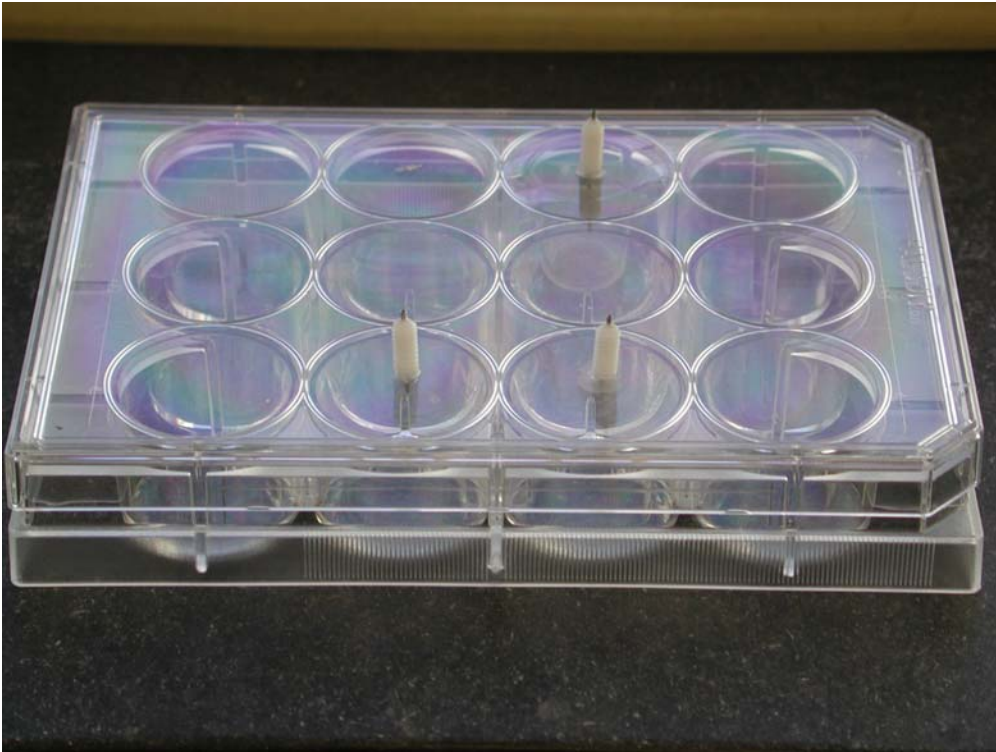
Figure 3. 12 well plate with vertically placed guide cannulae. Collagen gel was made in cell culture inserts, which were then placed in the plate. Tip of the 25-gauge syringe needle passed through one of the guide cannula into collagen gel.
