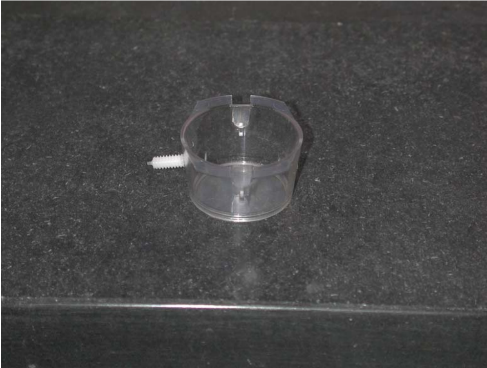
Figure 5. Cell culture insert with laterally implanted guide cannula. The cell culture insert with the cannula was placed in a 6 well plate. Cell suspension was drawn in a needle and tip of the 25-gauge syringe needle passed through the cannula into collagen gel. This assembly however resulted in poor cell delivery and growth and was not used for prototype catheter experiments.
