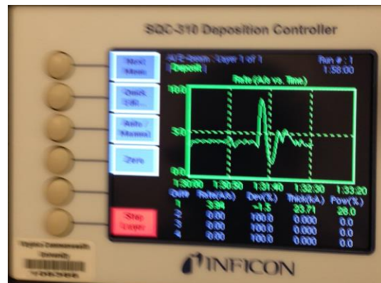
Figure 3.5: Deposition controller when the crucible is becoming empty, abnormal deposition rate and power percentage increased.
