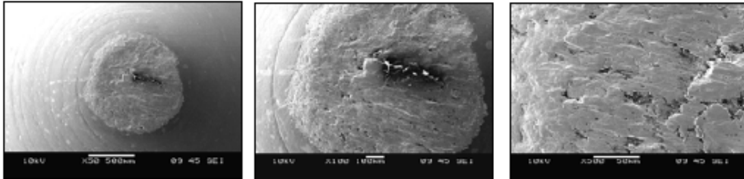
Figure 4.68 SEM picture at the tip of DC 53 die sample with TD coating (Sample # 4-2) with magnifications of a) 50X, b) 100X, c) 500X
