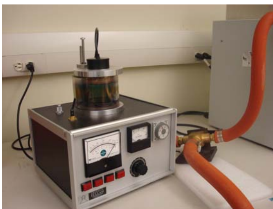
Figure 14. Sputter Coating Facility
