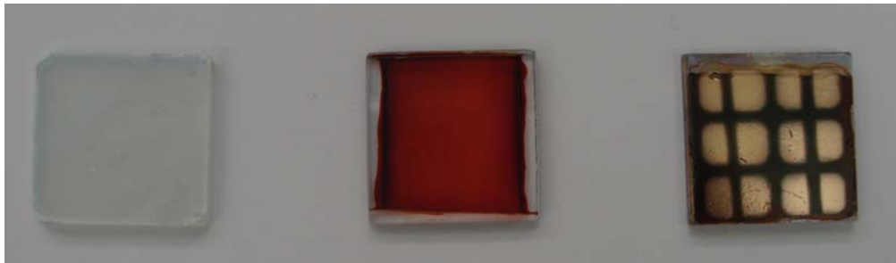
Figure 19. FTO substrates: left to right: (1) FTO square (2) Coated with PTEBS polymer (3) Sputter coated with gold electrodes
