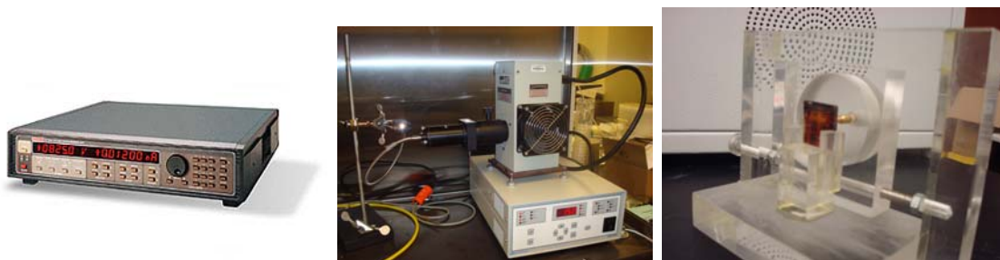
Figure 21. Current density-voltage measure system left to right (1) Keithley 236 source measure unit (2) Air Mass 1.5 illumination from Spectra-Physics Inc. (3) Tunable holding and testing instrument for solar cell I-V measurement.
