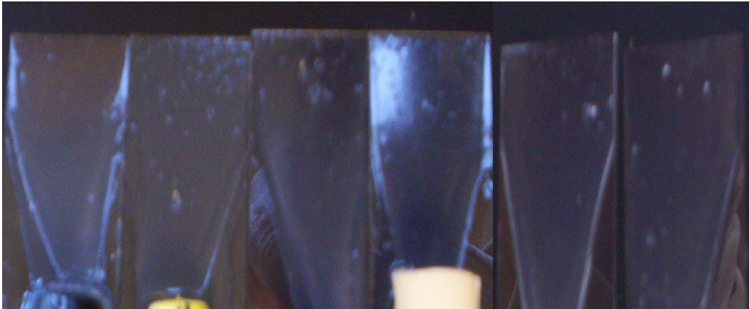
Figure 20. Cured solid dip coatings of 14 wt% uFSN in PDMS with 5.4 to 20.9 wt% (12.5x – 60x) crosslinker (L R) from Standard Heated Speed Mixing.
