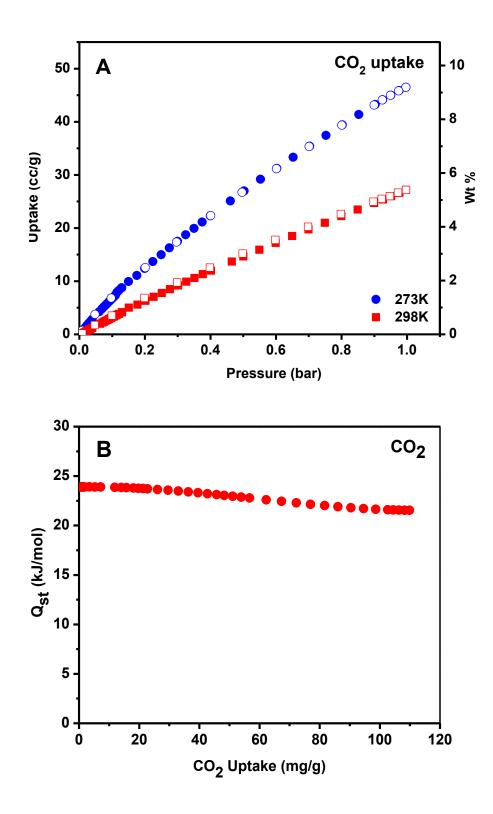
**Figure 2.13: A)** Carbon dioxide isotherm for *TDCOF-5* measured at 273K and 298K. **B)** Carbon dioxide isosteric heat of adsorption (*Qst*) for *TDCOF-5*.
