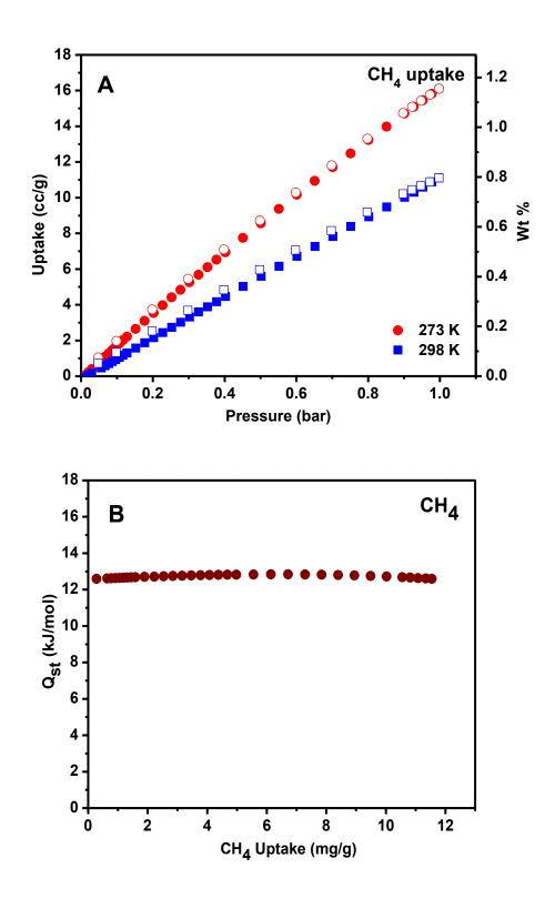
**Figure 2.12: A**) Methane isotherm for *TDCOF-5* measured at 273K and 298K. **B**) Methane isosteric heat of adsorption (*Qst*) for *TDCOF-5*.
