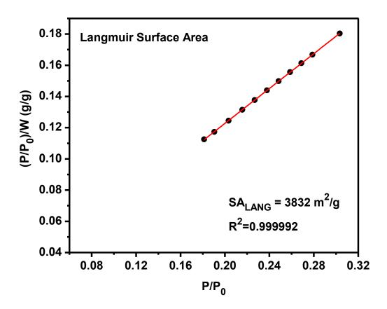
**Figure 2.8:** Langmuir plot for TDCOF-5 calculated from the Ar adsorption isotherm at 87 K. The model was applied from  $P/P_0 = 0.17$ -0.30. The correlation factor is indicated. (W= Weight of gas absorbed at a relative pressure  $P/P_0$ ).
