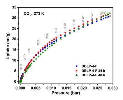
**Figure 4.9.** CO<sub>2</sub> isotherms for DBLP-4-F as synthesized, 24 h and 48 h exposed to air at 273K. The filled points are adsorption and the empty points are desorption.
