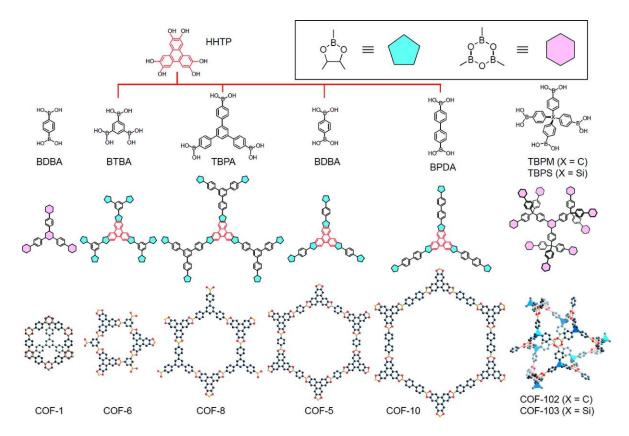
**Figure 1.6:** Formation of the COFs. Reprinted with permission from (FURUKAWA, H.; YAGHI, O. M., STORAGE OF HYDROGEN, METHANE, AND CARBON DIOXIDE IN HIGHLY POROUS COVALENT ORGANIC FRAMEWORKS FOR CLEAN ENERGY APPLICATIONS. J. AM. CHEM. SOC. 2009, 131, (25), 8875-8883.). Copyright (2009) American Chemical Society.
