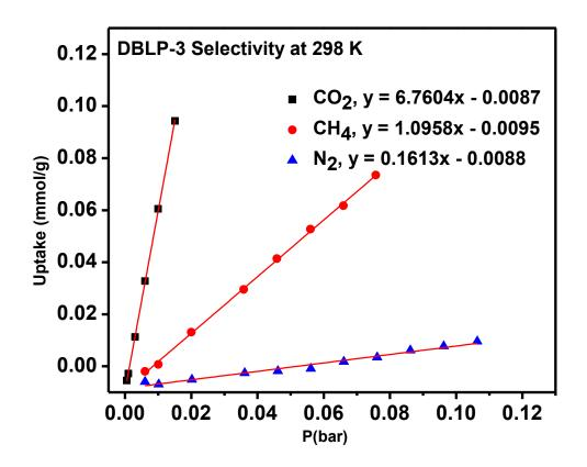
**Figure 3.30:** Adsorption selectivity of  $CO_2$  over  $N_2$  and  $CH_4$  for DBLP-5 from initial slope calculations.  $CO_2$  (black),  $CH_4$  (red) and  $N_2$  (blue) isotherms collected at and 298 K.
