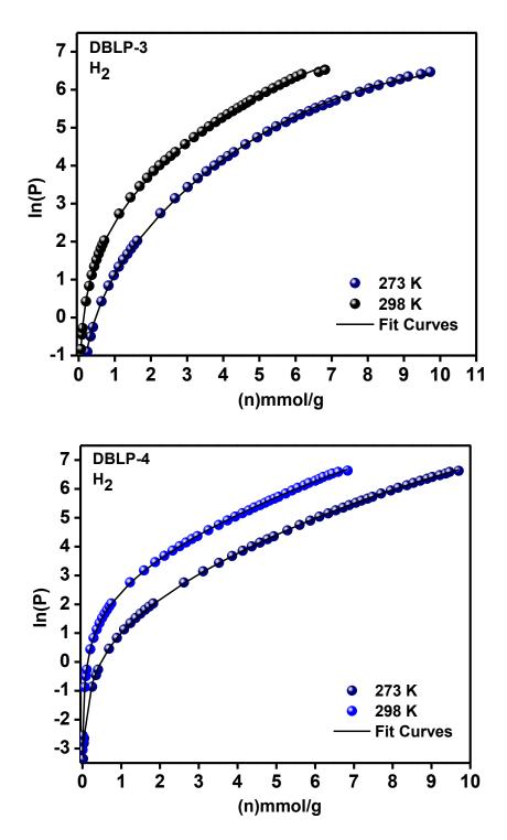
Figure 3.22: Virial analysis of H<sub>2</sub> adsorption data for DBLP-3, and DBLP-4.
