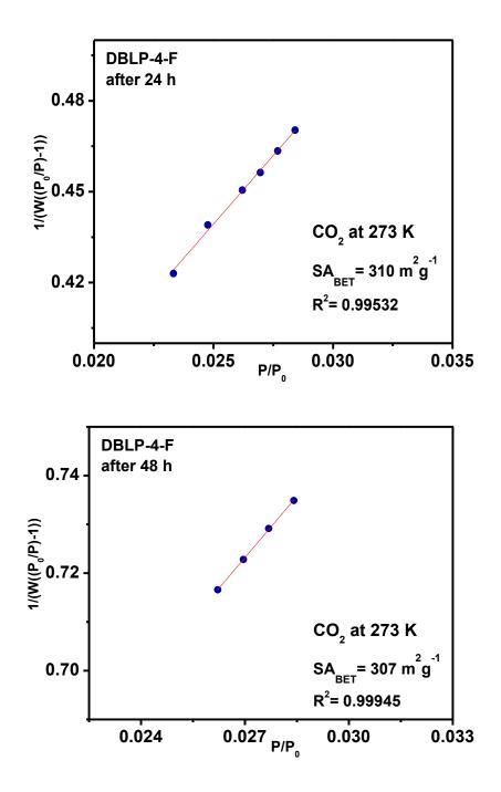
**Figure 4.11.** Multipoint BET plots for DBLP-4-F, which are 24 h and 48 h exposed to air that are calculated from the CO<sub>2</sub> adsorption.
