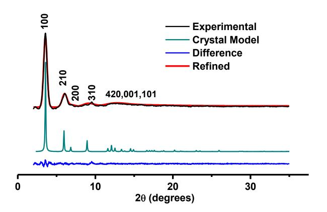
**Figure 2.16**: PXRD pattern of *TDCOF-5* with the experimental pattern in black, the Reitveld refined profile in red, the difference plot in blue and the eclipsed crystal model is green.
