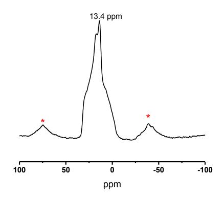
**Figure 2.2:** Solid-state <sup>11</sup>B multiple quantum MAS (MQMAS) NMR spectrum of TDCOF-5; asterisks denote spinning-side bands.
