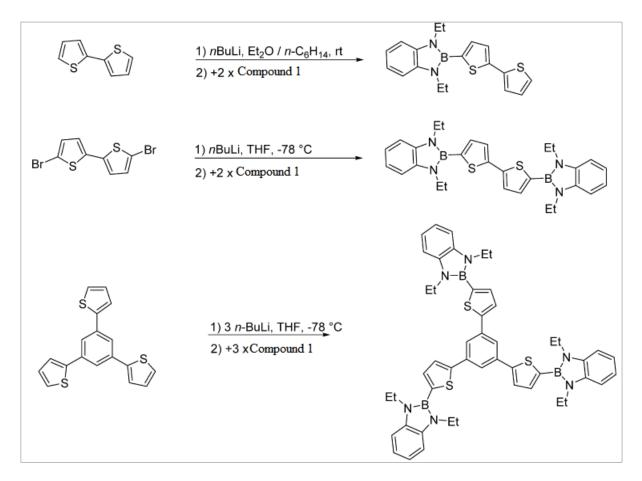
**Scheme 1.3:** Examples of 1,3,2-benzodiazaboroles synthesized by using organolithiums. Compound 1 is described in Scheme 1.2. Adapted from Ref. 7 with permission from Elsevier.
