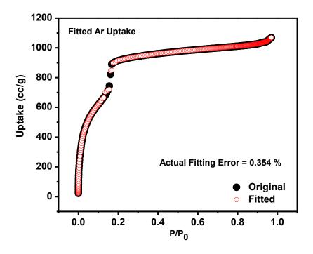
**Figure 2.7:** Experimental Ar adsorption isotherm for TDCOF-5 measured at 87 K is shown as filled circle. The calculated NLDFT isotherm is overlaid as open circle. Note that a fitting error of less than 1% indicates the validity of using this method for assessing the porosity of TDCOF-5. The fitting error is indicated.
