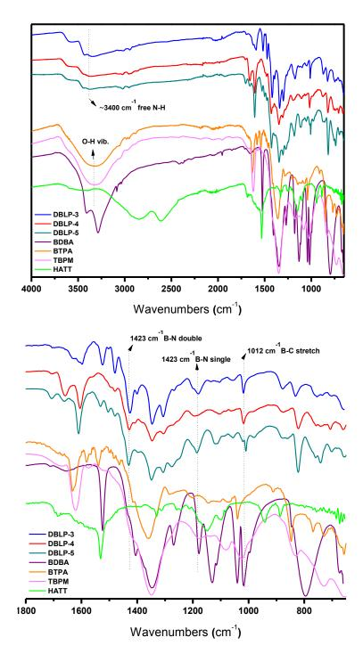
**Figure 3.1:** FT-IR spectra of DBLPs and their starting building units. Lower panel is an expanded region from 600 to 1800 cm<sup>-1</sup>
