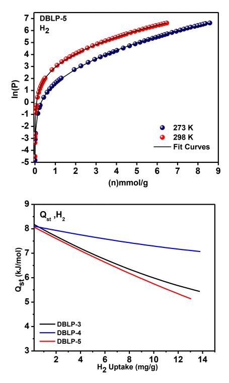
**Figure 3.23:** Virial analysis of H<sub>2</sub> adsorption data for DBLP-5 and the isosteric heat of adsorption ( $Q_{st}$ ) for DBLP-3, DBLP-4, and DBLP-5.
