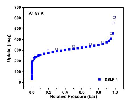
**Figure 4.6.** Argon isotherm for DBLP-4 measured at 87 K. The filled squires are adsorption points and the empty squires are desorption points.
