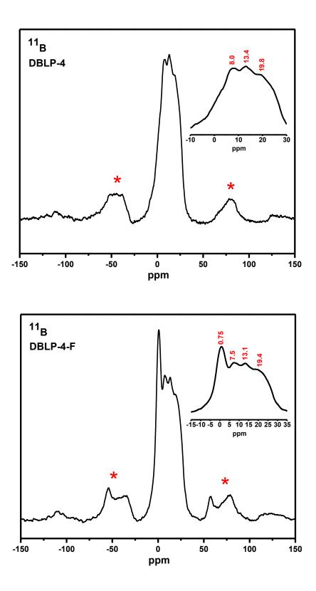
**Figure 4.3.** Solid-state <sup>11</sup>B multiple quantum MAS (MQMAS) NMR spectrum of DBLP-4 and DBLP-4-F; asterisks denote spinning-side bands.
