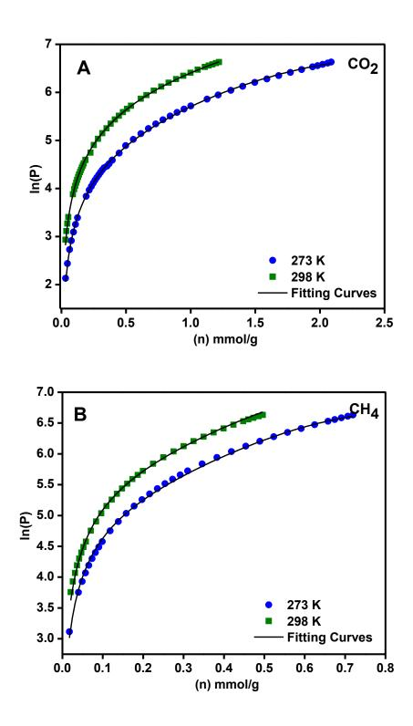
Figure 2.15: Virial analysis of A) CO<sub>2</sub> and B) CH<sub>4</sub> adsorption data for *TDCOF-5*
