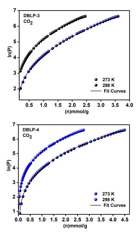
Figure 3.20: Virial analysis of CO<sub>2</sub> adsorption data for DBLP-3, and DBLP-4.
