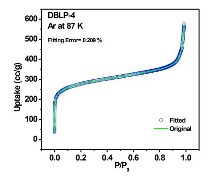
**Figure 4.7.** NLDFT calculated isotherm for DBLP-4 overlaid with the experimental argon isotherm. A fitting error less than 1% indicates validity of the model.
