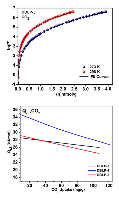
**Figure 3.21:** Virial analysis of CO<sub>2</sub> adsorption data for DBLP-5 and the isosteric heat of adsorption ( $Q_{st}$ ) for DBLP-3, DBLP-4, and DBLP-5.
