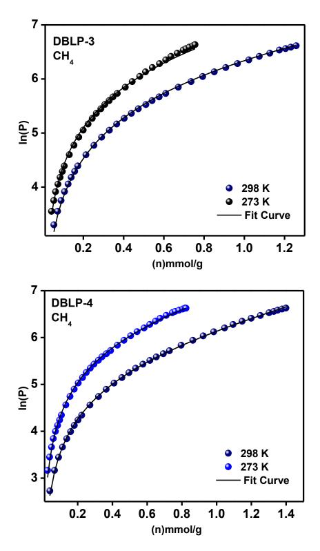
Figure 3.24: Virial analysis of CH<sub>4</sub> adsorption data for DBLP-3, and DBLP-4.
