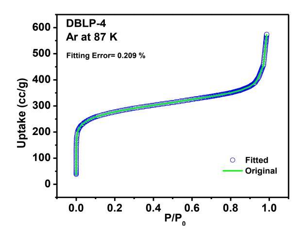
**Figure 3.10:** Experimental Ar adsorption isotherm for DBLP-4 (blue) measured at 87 K. The calculated NLDFT isotherm is overlaid as open circle. Note that a fitting error of < 1 % indicates the validity of using this method for assessing the porosity of DBLPs. The fitting error is indicated.
