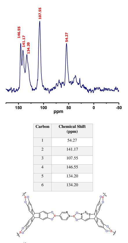
Figure 2.4: Solid-State <sup>13</sup>C CP-MAS NMR spectrum for TDCOF-5.
