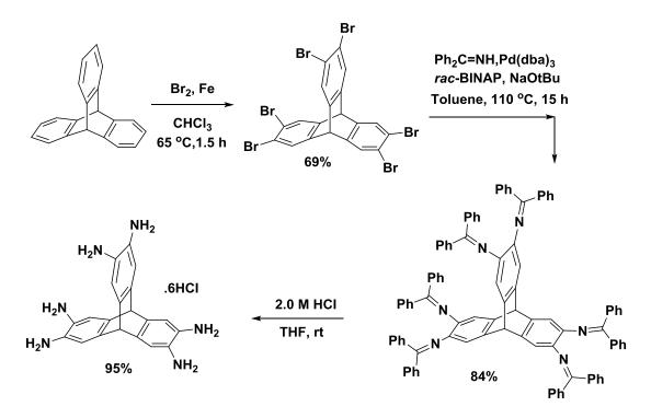
Scheme 3.1: Overall synthesis of hexahydroxytriptycene and haxaaminotriptycene (HCl salt)
