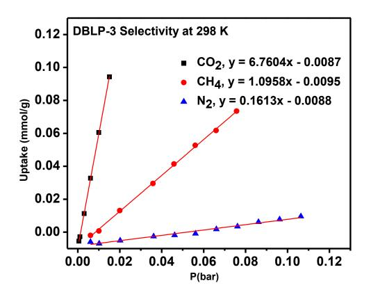
**Figure 3.28:** Adsorption selectivity of  $CO_2$  over  $N_2$  and  $CH_4$  for DBLP-3 from initial slope calculations.  $CO_2$  (black),  $CH_4$  (red) and  $N_2$  (blue) isotherms collected at and 298 K.
