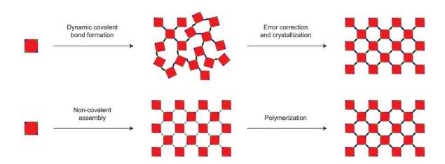
**Figure 1.5:** Schematic illustrations of the error correction step. This figure used with the permission from Nature Publishing Group. <sup>11</sup>
