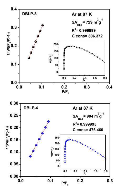
**Figure 3.14:** BET plot for DBLP-3 (black), and DBLP-4 (blue) calculated from the Ar adsorption isotherm at 87 K. The model was applied from  $P/P_0$ = 0.04-0.16. The correlation factor is indicated. (W= Weight of gas absorbed at a relative pressure  $P/P_0$ ).
