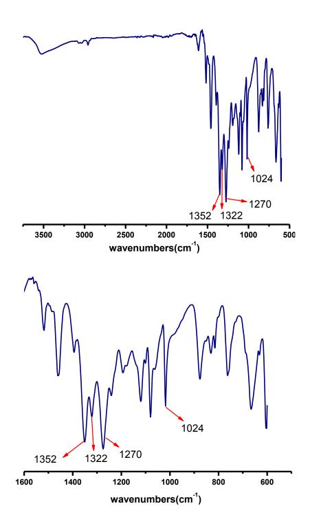
**Figure 2.1:** FT-IR spectra were obtained as KBr pellets using a Nicolet Nexus 670 FT-IR spectrometer. The formation of the  $BC_2O_2$  ring is supported by the following IR-bands (cm-1): B-O (1352), B-C (1270), and C-O (1024). FT-IR results are in line with previous reported COFs. <sup>1-4</sup>
