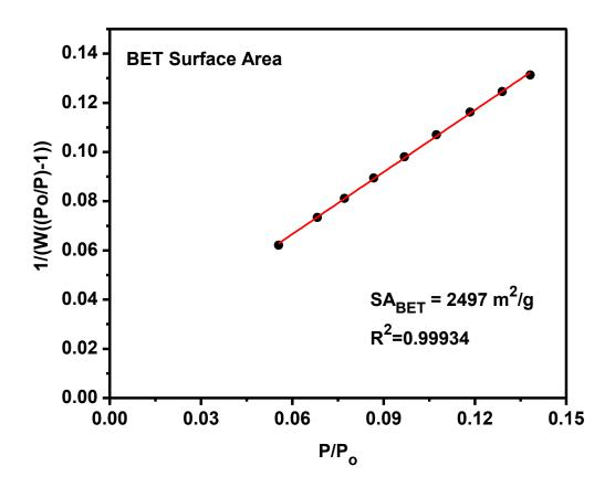
**Figure 2.9:** BET plot for TDCOF-5 calculated from the Ar adsorption isotherm at 87 K. The model was applied from  $P/P_0 = 0.05 \cdot 0.15$ . The correlation factor is indicated. (W= Weight of gas absorbed at a relative pressure  $P/P_0$ ).
