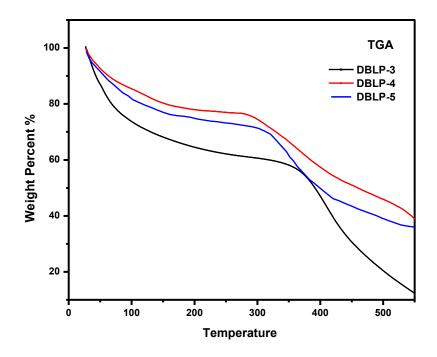
Figure 3.4: Thermogravimetric analysis of DBLPs
