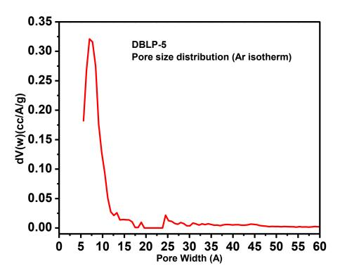
**Figure 3.13:** Pore Size Distribution for DBLP-5 (red) was calculated from the Ar adsorption isotherms by the Non-Local Density Functional Theory (NLDFT) method using a cylindrical pore model.
