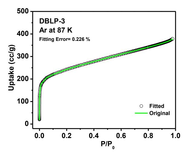
**Figure 3.9:** Experimental Ar adsorption isotherm for, DBLP-3 (black) measured at 87 K. The calculated NLDFT isotherm is overlaid as open circle. Note that a fitting error of < 1 % indicates the validity of using this method for assessing the porosity of DBLPs. The fitting error is indicated.
