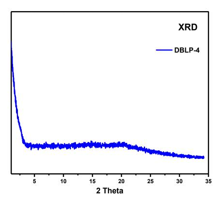
**Figure 4.5.** Powder X-ray Diffraction Analysis of DBLP-4: Powder X-ray diffraction data of DBLP-4 were collected on a Panalytical X'pert Pro Multipurpose Diffractometer (MPD). Samples were mounted on a zero background sample holder measured in transmission mode using Cu K $\alpha$  radiation with a 2 $\theta$  range of 1.5-35°.
