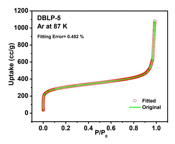
**Figure 3.11:** Experimental Ar adsorption isotherm for DBLP-5 (red) measured at 87 K. The calculated NLDFT isotherm is overlaid as open circle. Note that a fitting error of < 1 % indicates the validity of using this method for assessing the porosity of DBLPs. The fitting error is indicated.
