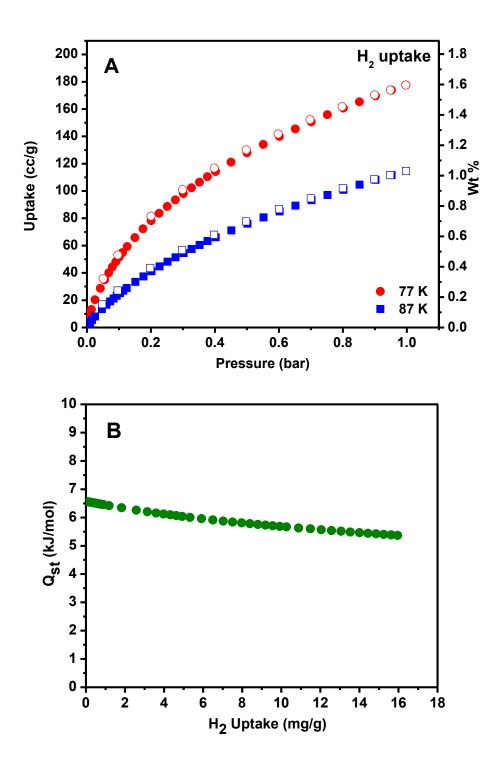
**Figure 2.11: A)** Hydrogen isotherm for *TDCOF-5* measured at 77K and 87K. **B)** Hydrogen isosteric heat of adsorption (*Qst*) for *TDCOF-5*.
