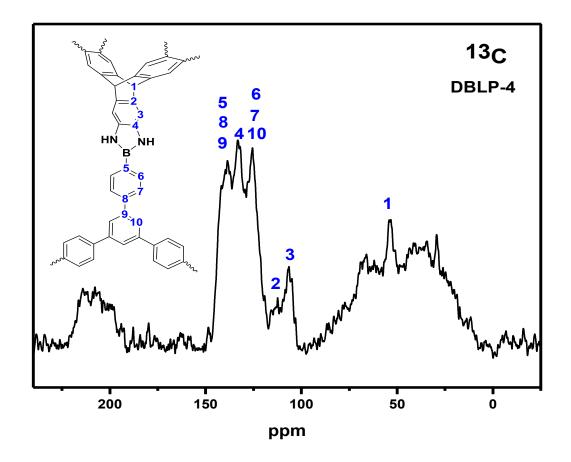
Figure 4.1. Solid-State <sup>13</sup>C CP-MAS NMR spectrum for DBLP-4.
