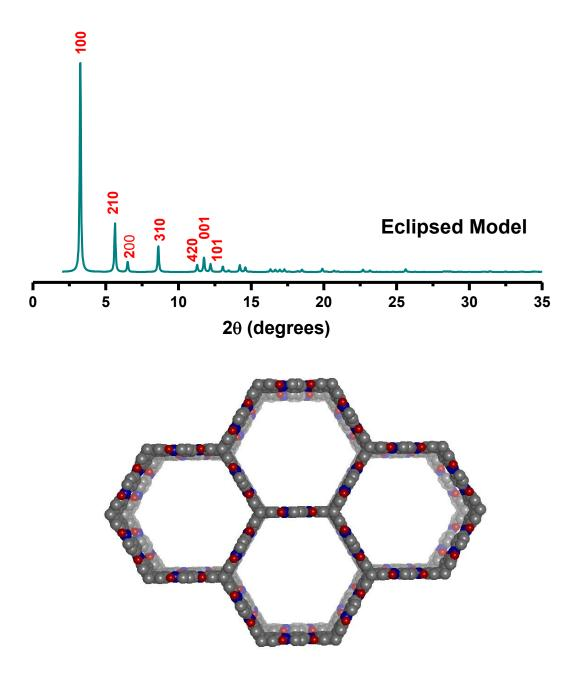
Figure 2.17: Eclipsed PXRD pattern of *TDCOF-5*
