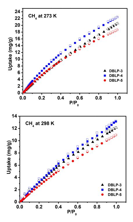
**Figure 3.19:** CH<sub>4</sub> uptake isotherms for DBLP-3 (black), DBLP-4 (blue) and DBLP-5 (red) at 273 and 298 K.
