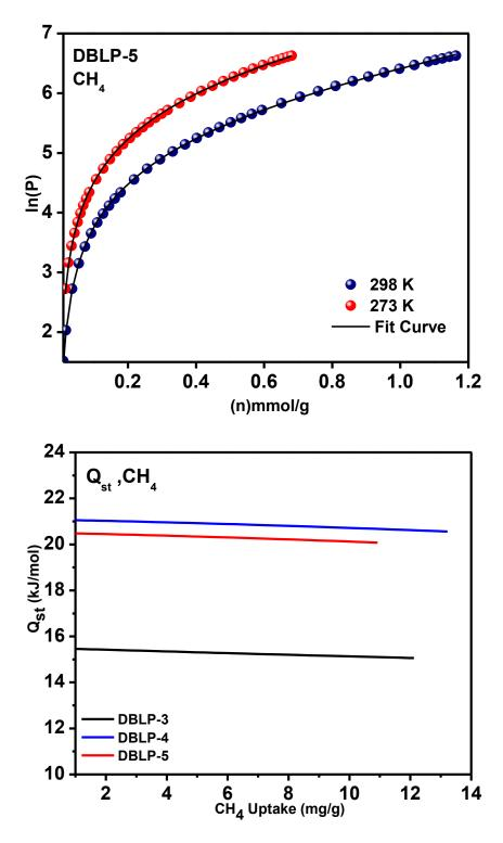
**Figure 3.25:** Virial analysis of CH<sub>4</sub> adsorption data for DBLP-5 and the isosteric heat of adsorption ( $Q_{st}$ ) for DBLP-3, DBLP-4, and DBLP-5.
