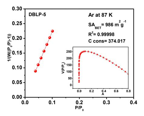
**Figure 3.15:** BET plot for DBLP-5 (red) calculated from the Ar adsorption isotherm at 87 K. The model was applied from  $P/P_0= 0.04-0.16$ . The correlation factor is indicated. (W = Weight of gas absorbed at a relative pressure  $P/P_0$ ).
