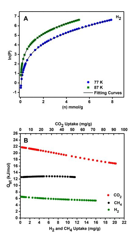
**Figure 2.14: A**) Virial analysis of H<sub>2</sub> adsorption data for *TDCOF-5*. **B**) Combined isosteric heat of adsorption (*Ost*) for *TDCOF-5*.
