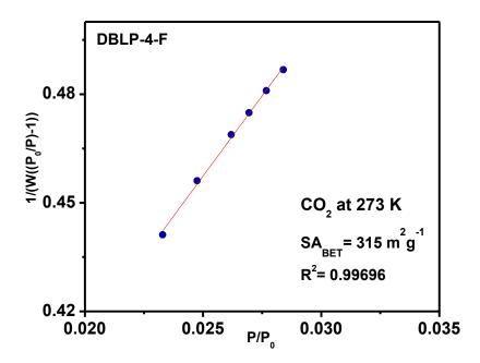
Figure 4.10. Multipoint BET plots for DBLP-4-F as synthesized calculated with CO<sub>2</sub> at
