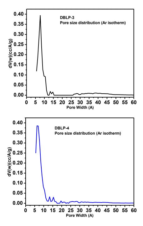
**Figure 3.12:** Pore Size Distribution for DBLP-3 (black) and DBLP-4 (blue) was calculated from the Ar adsorption isotherms by the Non-Local Density Functional Theory (NLDFT) method using a cylindrical pore model.
