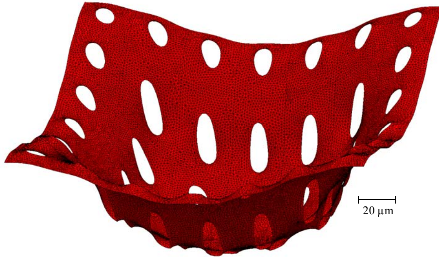
Figure 3.11: Equilibrium meniscus shape and position for the structure from Figure 3.10 solved through minimization of interfacial energy. Area-averaged meniscus height is equal to -3.528 \mu\text{m} , less than 5% error with Equation 3.1. The array has a SVF of 0.1, and a unimodal fiber diameter of 10 \mu\text{m} . The outside fibers have a water contact angle of 60^\circ , and the inside fibers a water contact angle of 120^\circ .
