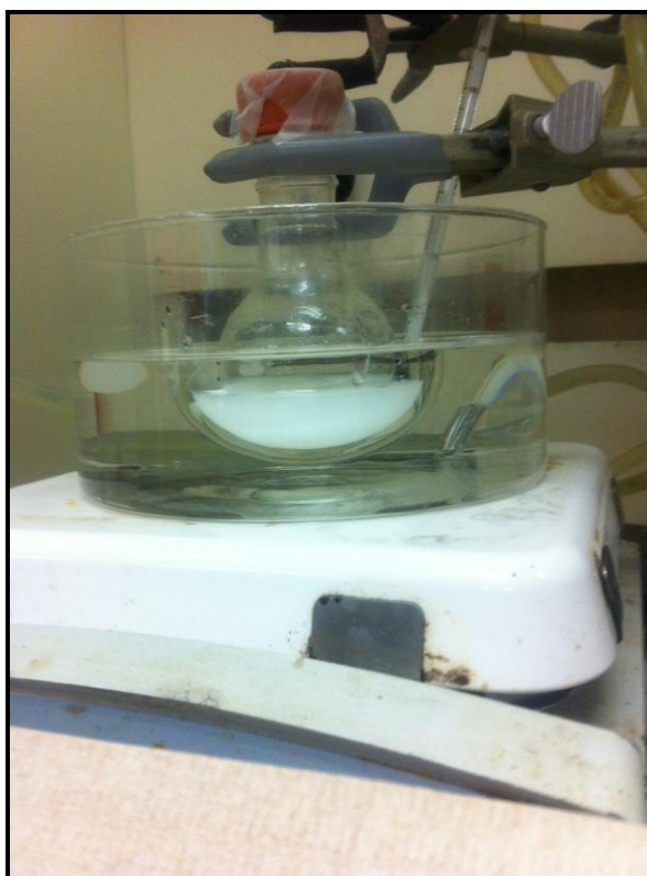
Figure 20: Milky white reaction mixture signalling the end of the polymerization reaction
