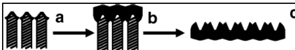
Figure 8: Schematic diagram of preparation of silver porous film using anodized aluminum as a template.
