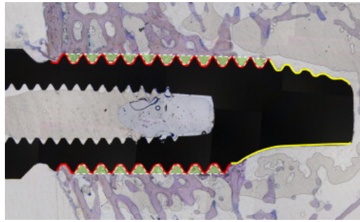
Fig. 2. Roughness of bone-to-implant contact is strongly and positively correlated to bone healing (within some range of roughness).
