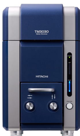
Fig. 27. Benchtop Scanning Electron Microscope, model TM3030 (by Hitachi) used to produce micrographs of ablated surfaces. Equipment located in the Wright Center Laboratory at the Virginia Commonwealth University.
