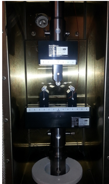
Fig. 33. Insight 30 MTS machine used to carry out flexural tests. Equipment located in the east building of the Department of Mechanical and Nuclear Engineering at the Virginia Commonwealth University.
