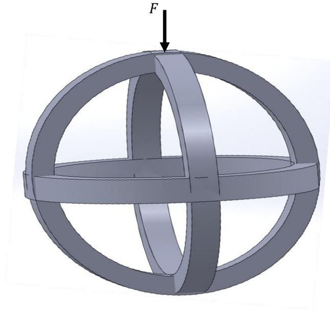
Fig. 5.4 An external perpendicular force F applied to deform the bladder and change the shape.
