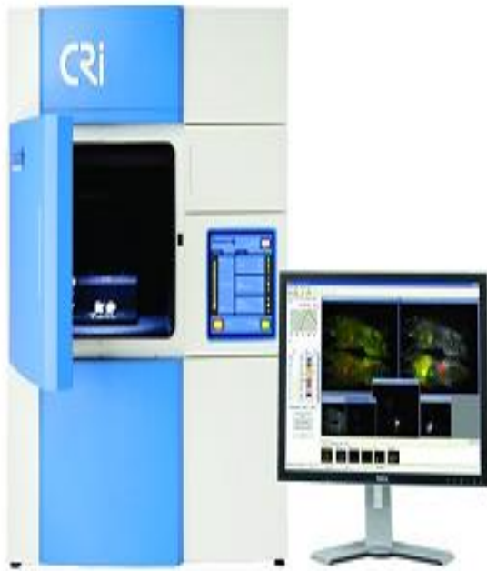
Figure 7 Multispectral fluorescence imaging system (Maestro2 at CMI/VCU). Wavelength range = 500-950 nm; FOV = Max 3 mice; Spectral Unmixing and Dynamic Contrast Enhancement (DyCE™) allows quantitation of temporal biodistribution of fluorescent markers at much earlier time points (first few seconds following injection).
