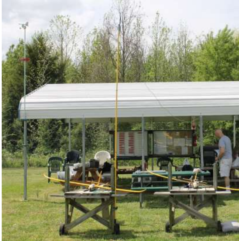
Fig 3.4. The field antenna and GCS node mounted on 10 ft. pole
