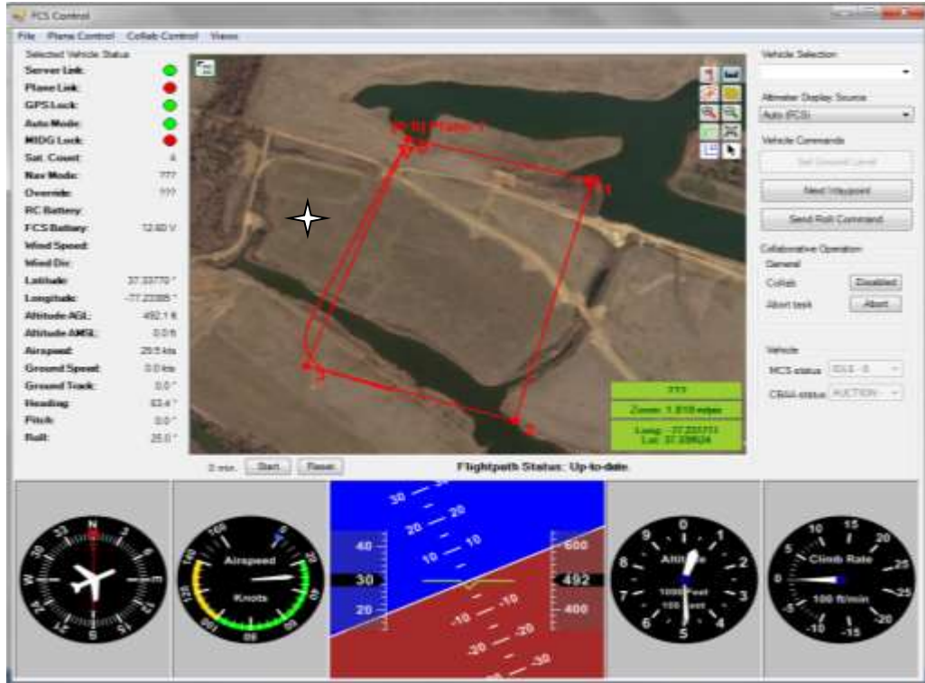
Fig 5.9. The set of waypoints 0, 1, 2 and 3 (red) assigned to the UAV in the real-world and simulation to validate the propagation loss model
