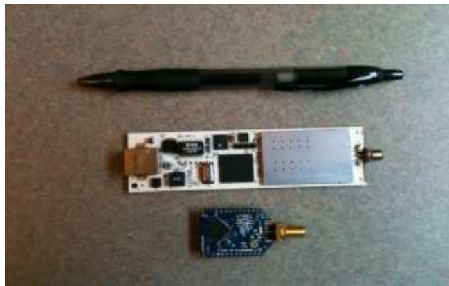
Fig 3.1. The modified bullet5 modem having the N-type connect replaced by RP-SMA
