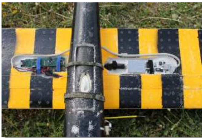
Fig 3.3. Physical location of wireless modem (right) inside UAV
