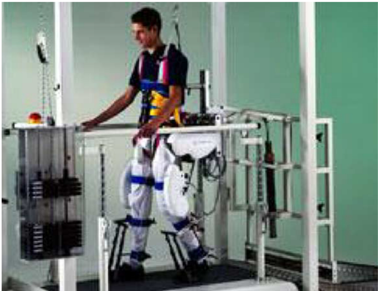
Figure 1 Lokomat™ Robotic Gait trainer is expensive, has limited availability, and less than ideal joint kinematics
