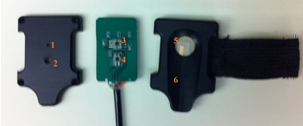
Figure 13: The real prototype device. Features: (1) pinhole aperture, (2) push-button opening, (3) RGB sensor, (4) push-button switch, (5) piezo-actuator, and (6) groove for the finger.
