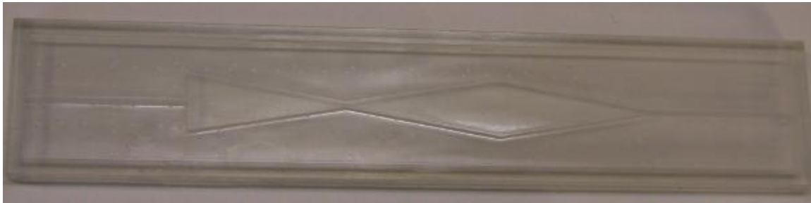
Figure 3.33: Rapid Prototyped PDMS Micropump Mold
