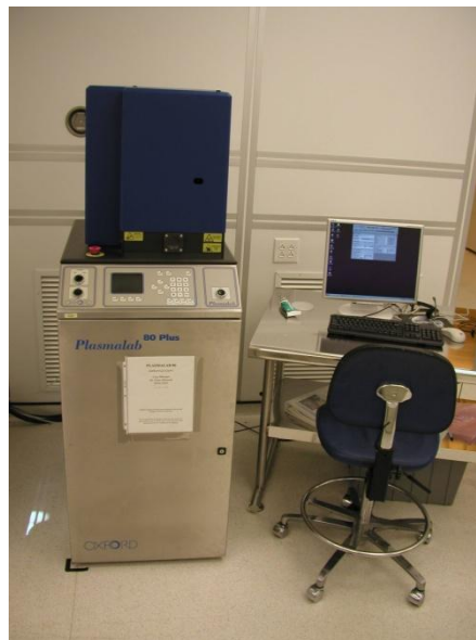
Figure 3.57: Plasmalab 80 Plus utilized for Sealing PDMS
