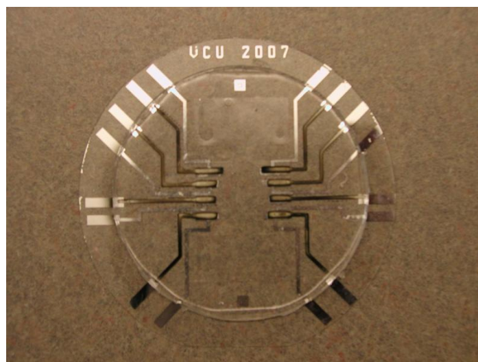
Figure 3.25: Complete Fabricated Electrostatic Actuated PDMS Micropump
