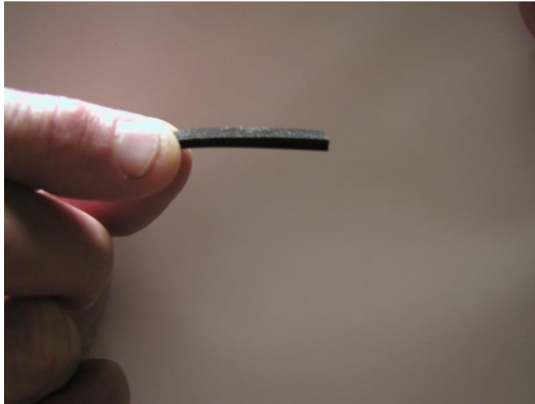
Figure 4.5: Magnetic PDMS Pump prior to Magnet Application (side view)
