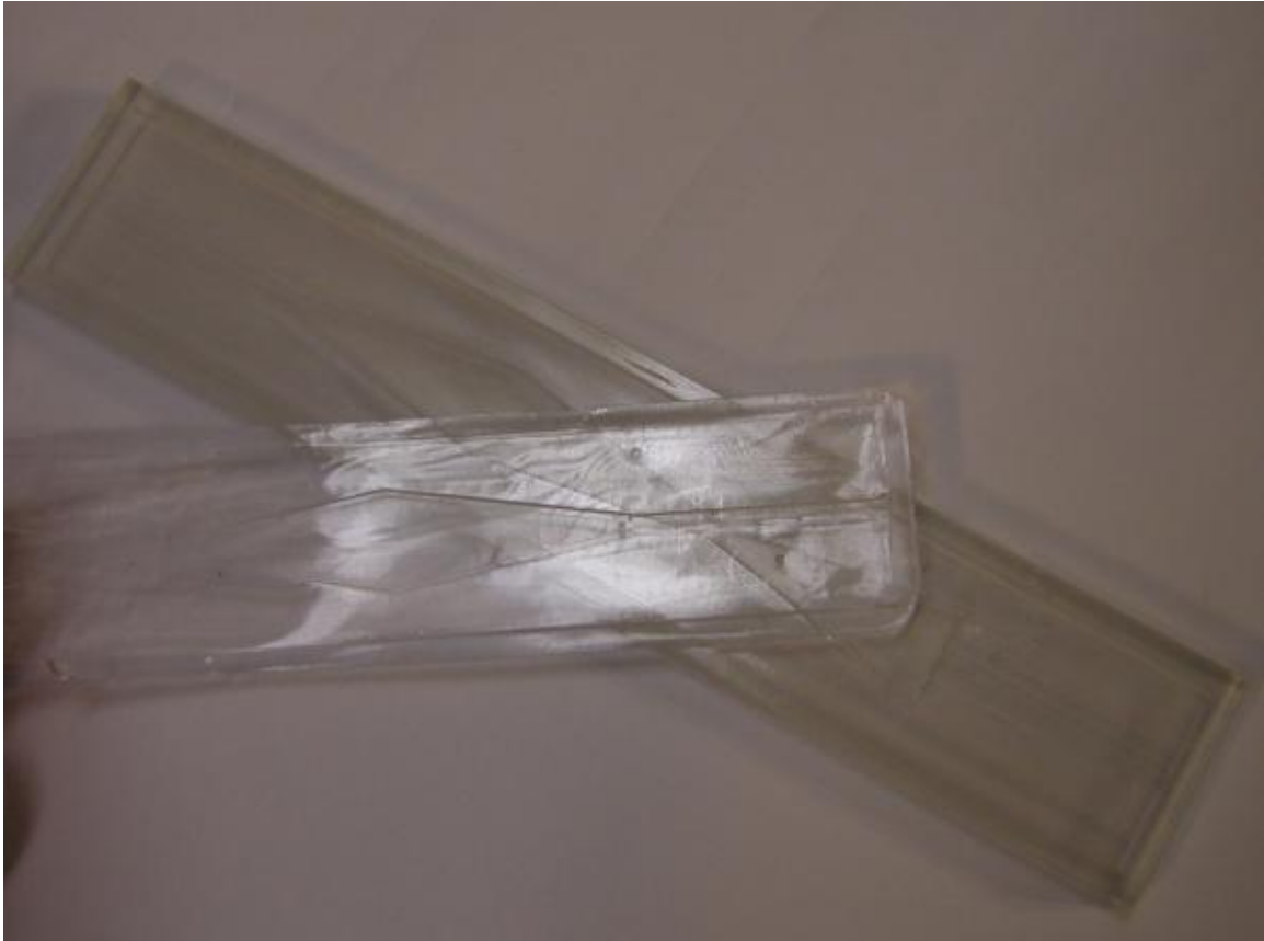
Figure 3.35: PDMS Completely Removed from Mold
