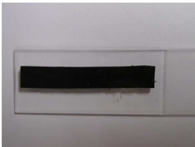
Figure 4.8: Magnetic Micropump Sealed to Substrate
