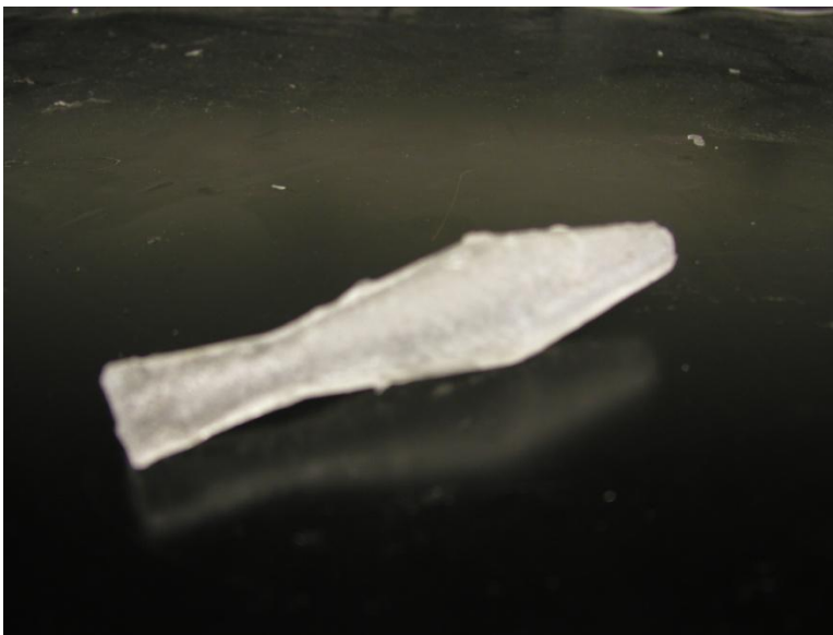
Figure 5.15: Three-dimensional micropump Fabricated
