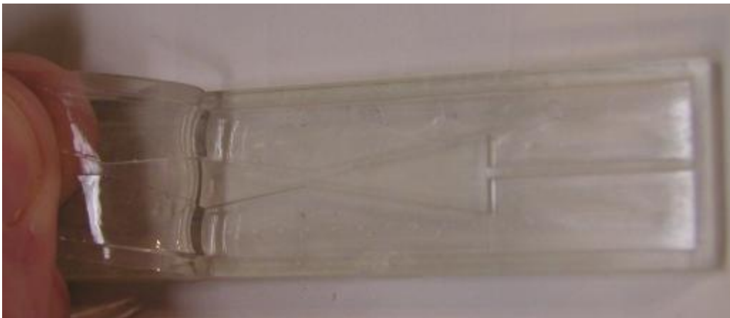
Figure 3.34: Removing PDMS from Mold
