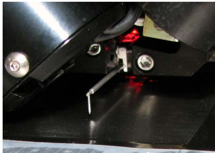
Figure 3-7 Stylus profiler (Ambios XP1).
