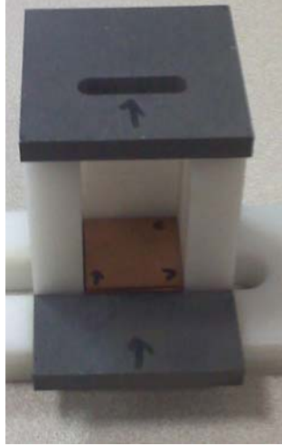
Figure 2: The attenuation measurement collimator assembly used for equivalent spectrum fitting. Stacks of high purity Al and Cu filters are placed in the phantom. The lead collimators are \frac{1}{4} " thick to block scattered radiation. The collimator opening is \frac{1}{4} " wide allowing approximately 5 to 6 detectors to be irradiated per view, and \frac{3}{4} " long in the z-direction allowing approximately 400 views to be acquired as the table translates in surview mode.
