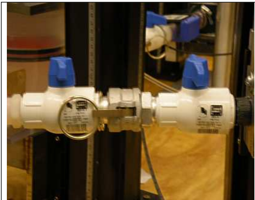
Figure 3.3. Mock loop quick disconnect mechanism.
