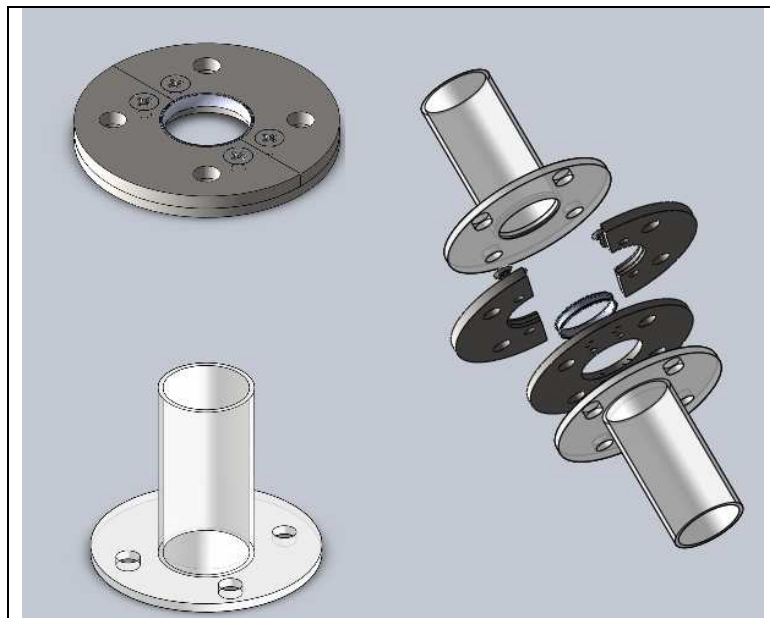
Figure 3.4. SolidWorks models of 25mm valve collar (top left), inlet/outlet MHV testing chamber (bottom left), and exploded view of MHV testing chamber assembly (right).
