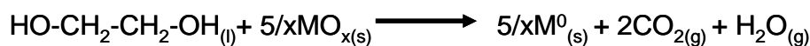
Figure 7.4. Proposed mechanism for the formation of Metal nanoparticles from metal oxide precursors. The reaction assumes that a complete oxidation of ethylene glycol produces gaseous carbon dioxide and water.
