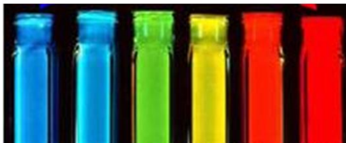
Figure 1.3. Fluorescence emission of CdSe(ZnS) quantum dots of various sizes(image is adapted from reference). 46
