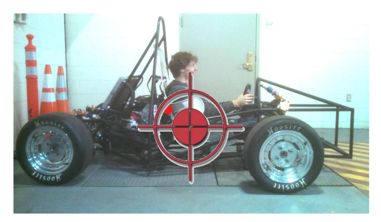
The Bull's-eye marks the center of gravity of the racecar. When we hit the brakes this moves forward and unloads the rear tires. What a mess this can make!
