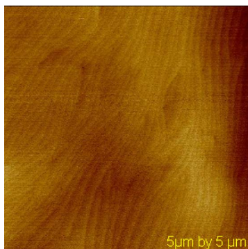
FIG. 2. (Color online) AFM image of a 10-nm-thick ZrO 2 on GaN. The image size is 5 \times 5 \mu\text{m}^2 and rms is 4 Å.
