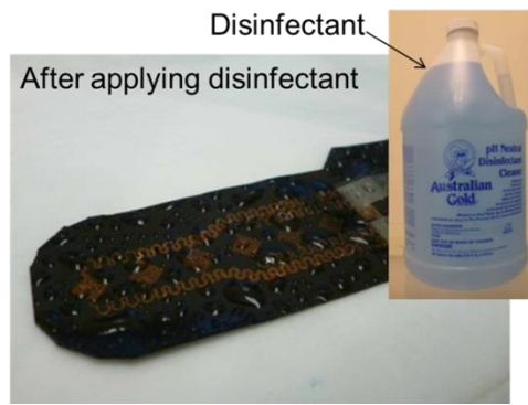
Figure S19. Photo of an EES after spraying with a disinfectant solution (pH Neutral Disinfectant Cleaner, Australian Gold, Indianapolis, IN, USA) for device cleaning.
