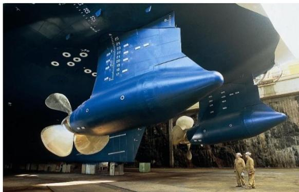
Foto 24: Hélice Azimutal. Fuente: [http://www.motorship.com/\\_\\_\\_data/assets/image/0009/726561/AZIPOD6\\_hi-2.jpg](http://www.motorship.com/___data/assets/image/0009/726561/AZIPOD6_hi-2.jpg)
