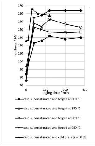
Figure 5 The influence of aging time on the hardness of pressed CuCrTiAl alloy.
