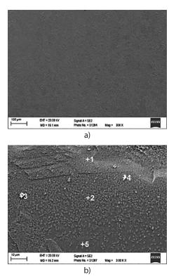
**Figure 6** Microstructure and EDS analysis of the CuCrTiAl alloy after hot deformation and aging at 480 °C for 2 hours, where the individual points have the following chemical composition (wt. %): 1. Cu-97,8, Cr-2,1, Al-0,1; 2. Cu-99,4, Cr-0,6; 3. Cu-5,1, Cr-82,4, Ti-3,2, P-9,2; 4. Cu-50,8, Cr-2,7, Ti-0,2, Al-26,2, O-20,1; 5. Cu-99,3, Cr-0,6, Al-0,1.
