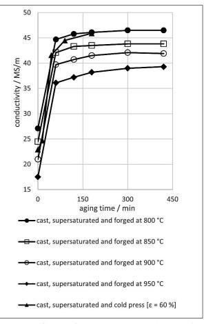
Figure 4 The influence of aging time on the conductivity of pressed CuCrTiAl alloy
