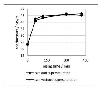
Figure 2 The influence of aging time on the conductivity of cast CuCrTiAl alloy.
