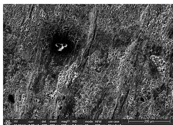
Figure 6 Metal burrs and impurities
