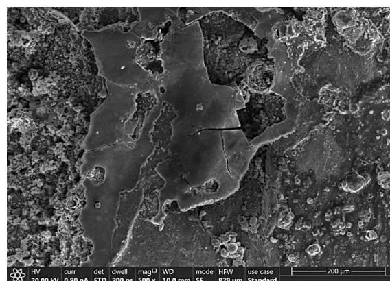
Figure 5 Corrosion product film-like morphology
