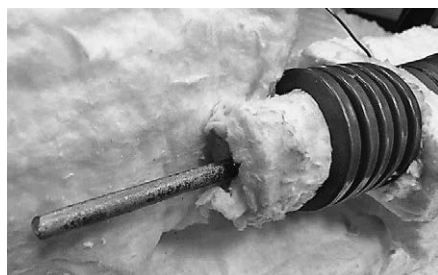
Figure 2 The view of the induction coil during the increasing temperature of the cast rod
