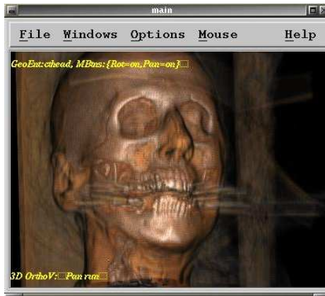
Figure 8: Rendering of a CT scan of the head of a cadaver. The beams projecting from the mouth are an artifact in the dataset, and are due to dental fillings scattering X-rays.
