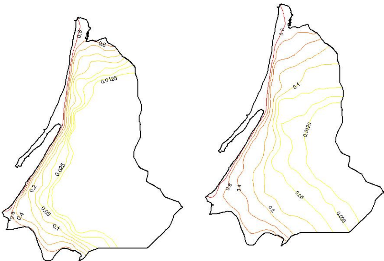
Figure 7: Thirty-year evolution of saltwater intrusion (normalized concentrations): contamination at 5 (left) and 30 (right) years.
