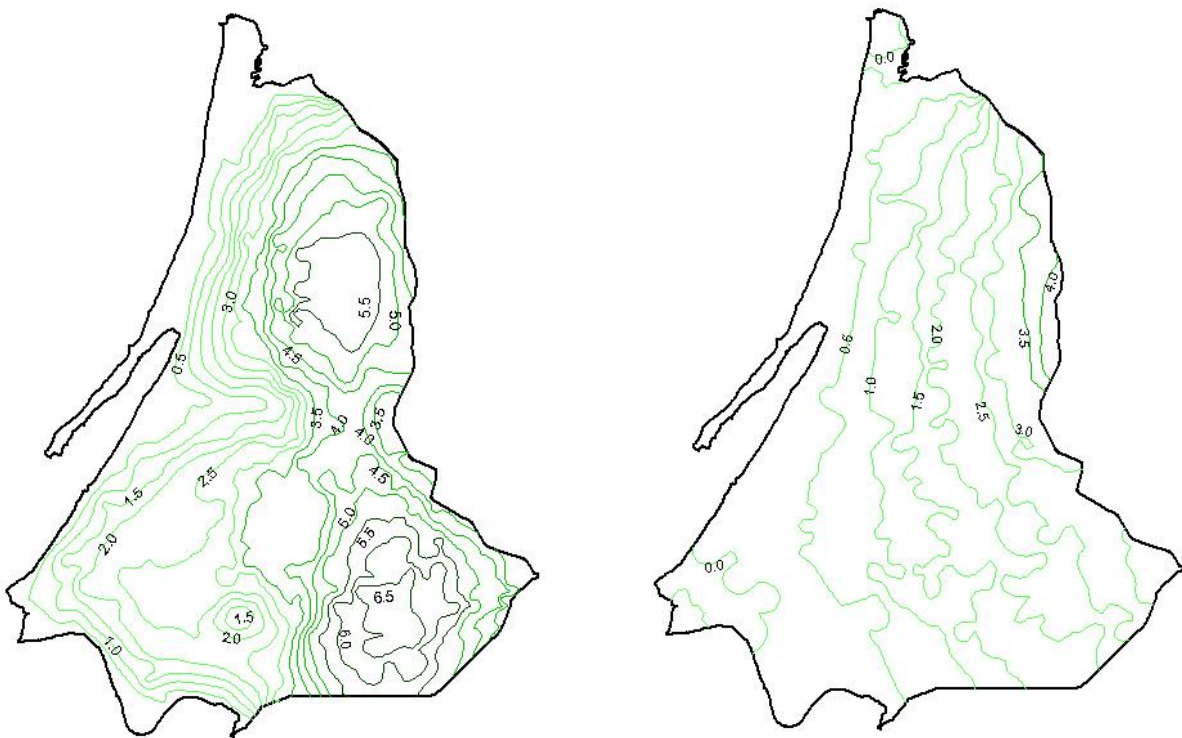
Figure 6: Calculated groundwater level contours (m) for the month of August (right) and December (left).
