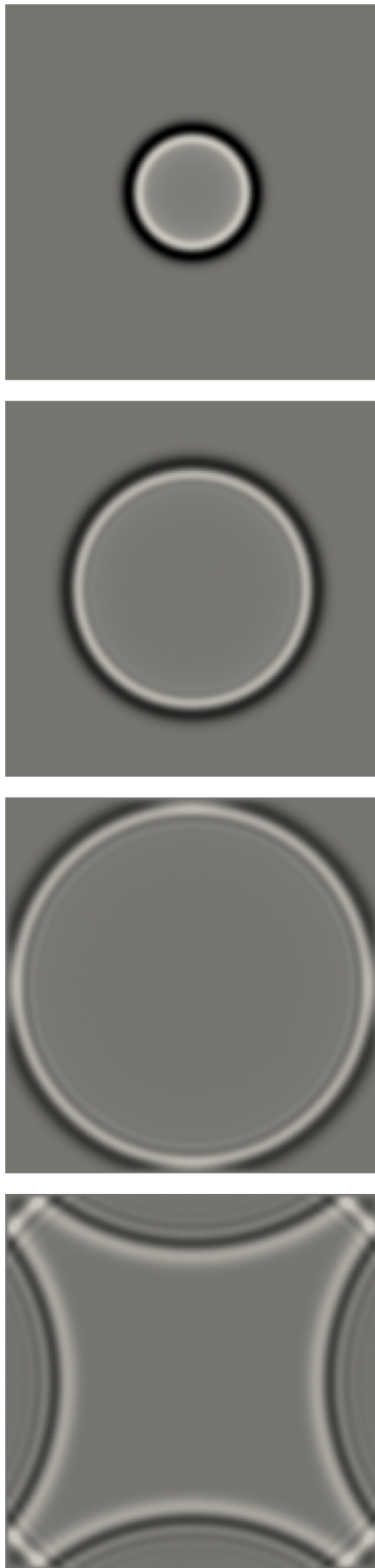
Fig. 3: Pressure wave test case: pressure wave propagation at 20, 40, 60, 80 \mu s
