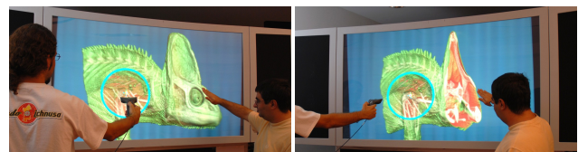
Fig. 1 Multi-user interactive exploration of a 64Gvoxel dataset on a 35Mpixel light field display. Users freely mix and match 3D tools creating view-dependent illustrative visualizations. Objects appear floating in the display workspace, providing correct parallax cues while delivering direction-dependent information.
