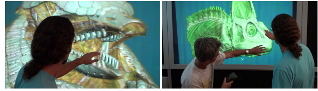
Fig. 13 Multi-user interactive exploration of 64Gvoxel datasets on a 35Mpixel light field display. Users freely mix and match 3D tools creating view-dependent illustrative visualizations. Objects appear floating in the display workspace, providing correct parallax cues while delivering direction-dependent information.
