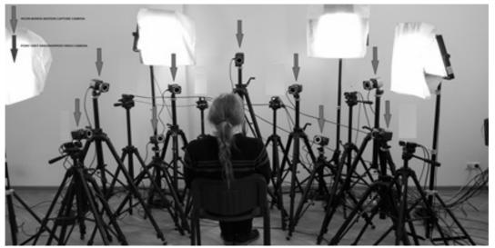
Figure 1. Placement of cameras around a patient in Human Facial Modelling Lab (arrows - Vicon Bonita cameras x10)
